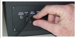
9. With volume control of TV/PC/Audio Device set at about 75% of maximum, turn up the volume of ZVOX Console all the way, or until audible distortion occurs. If distortion occurs, turn ZVOX volume control down until distortion goes away.
