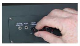
6. IMPORTANT: Turn down volume control on back panel of ZVOX Console to about the "9 o'clock" position.
