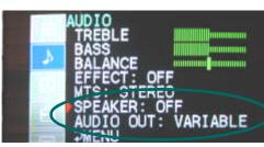
5. For TV connection only: All other devices, skip to step 6. If connected to a TV audio output, push the "MENU" button on your remote control, then choose "AUDIO" -- and navigate through the menu options to choose "SP EAKER: OFF" and "AUDIO OUT: VARIABLE" (sometimes called "AOV" on a TV's menu).
